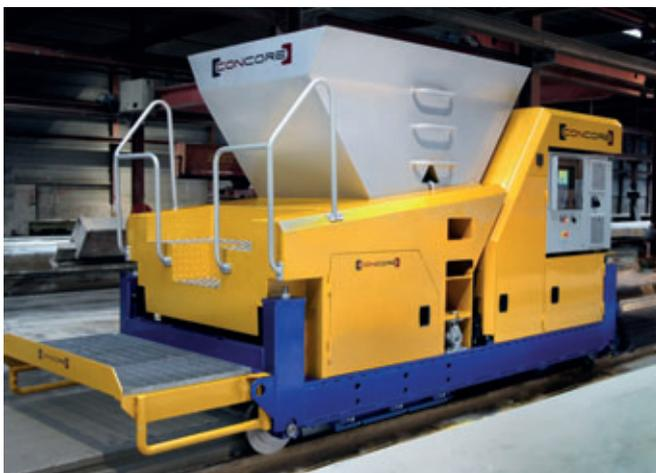
Fig. 1: Concore Standard Extruder
