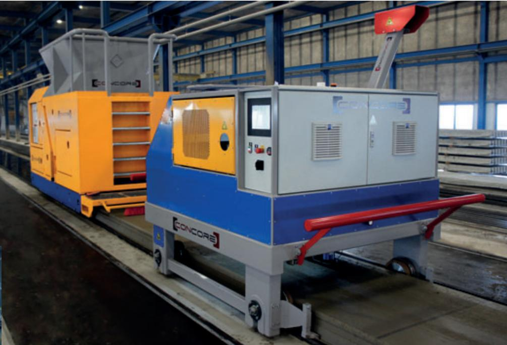
Fig. 3: A recent Concore delivery to a hollow-core slab factory with 6 beds in Bisofloor, the Netherlands. Concore modified the extruder to meet customer specifications.
